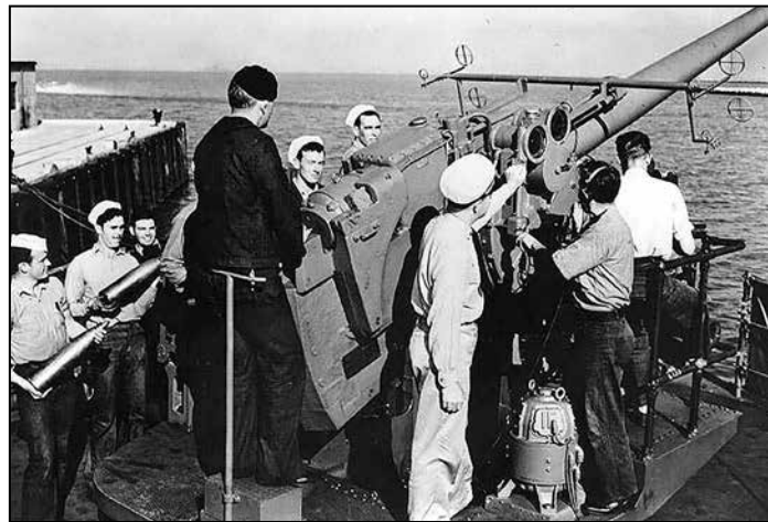
5"/38 caliber open mount gun aboard the USS Shaw (DD-373) in 1942. In addition to destroyers, the open-single mount was also installed on some civilian merchant ships but operated by U.S. Navy or Marine Corps gun crews. National Archives photo.
