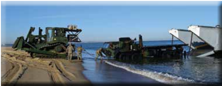
Sailors from Assault Craft Unit TWO (ACU2) work to remove a stuck Load Handling System (LHS) tactical truck from the shore with a bulldozer as part of their Joint Logistics Over-the-Shore (JLOTS) training with the U.S. Army at Fort Story, March 21, 2023. U.S. Navy photo by Lt. j.g. Michael F. Schwing.
