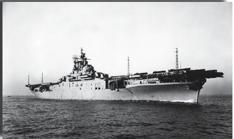
The USS Intrepid (CV-11), on her way to the Norfolk Navy Yard, back from her training cruise, 25 November 1943, Intrepid is seen passing Old Point Comfort at Hampton Roads. As completed, she had four tall lattice masts, supporting radio antennas, which could be hinged outboard during flight operations.
